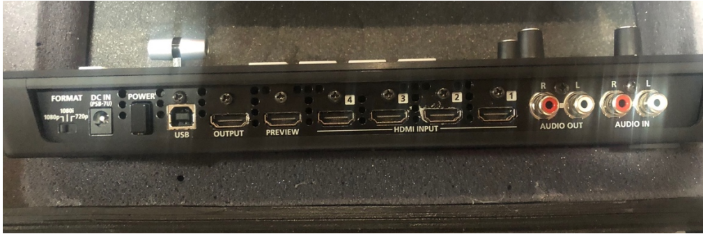
Figure 1 - HDMI Switcher - rear inputs
